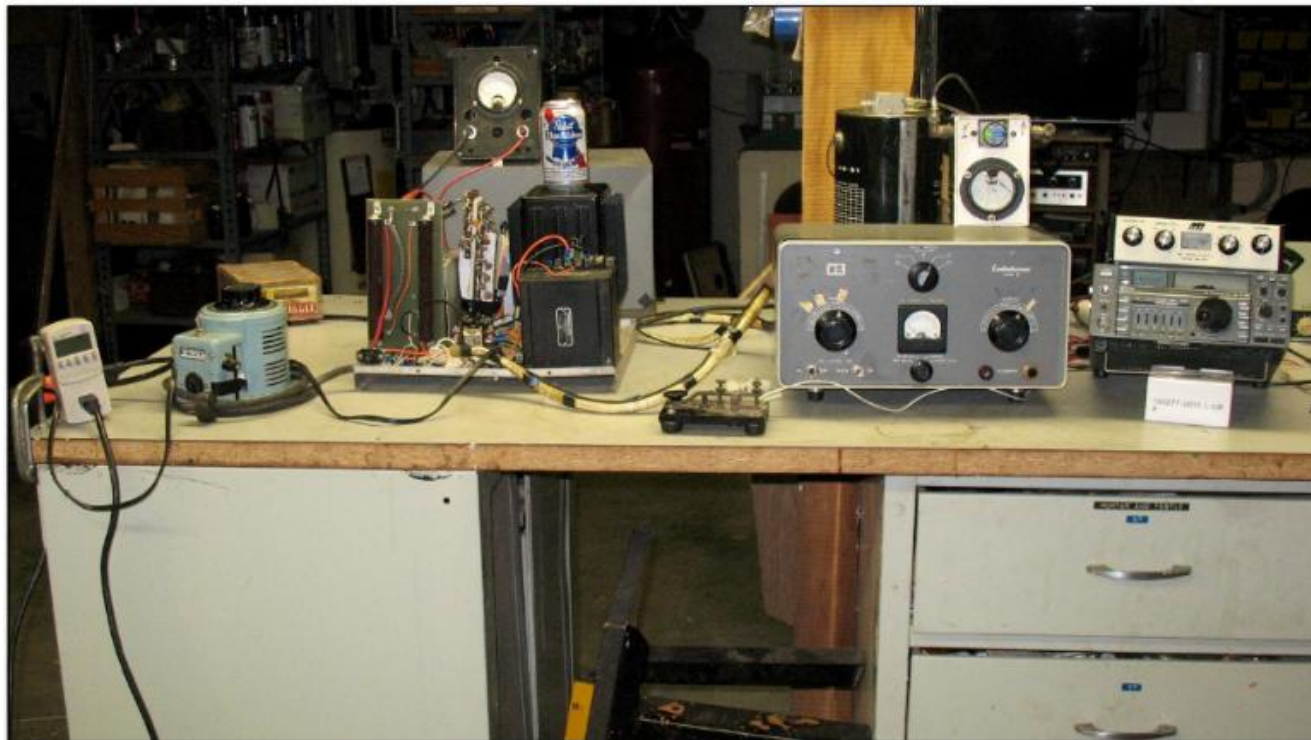
Picture 7 — Test setup on the bench. Comfortable operation seems to be a plate input of about 900W, which produces about 600W output, with about 50W drive from the IC-735 exciter. The Bird meter has been calibrated against Lowell's, so I think it's reasonably accurate.
