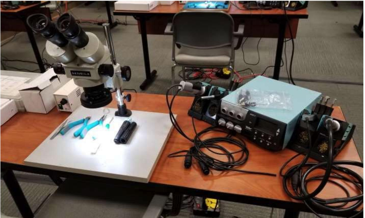
Weller soldering station with a microscope for surface mount parts.
