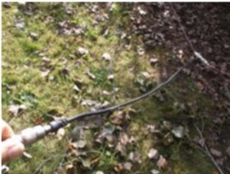
The length was calculated as  $(234/50.250) \times 0.66$  velocity factor = 3.07 feet. PL-259s were placed at each end of the Stub. Another F/F adapter connects the Stub to the RG-213 coax which goes to the shack.
