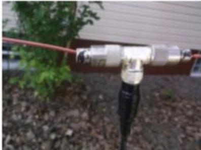
One end of the Delta loop is soldered to the center pin of one PL-259 and the other end of the loop is soldered to the outer case of the second PL-259. The two connectors are screwed into the T adapter. A Female to Female SO-239 connector is used to connect the T to the matching Stub coax.
