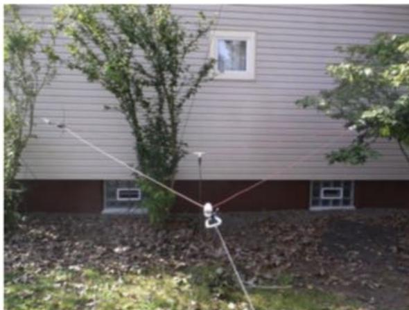
A 1/4 wave matching stub was made from RG59, 75 ohm coax. I did not have a 4:1 balun readily available.
