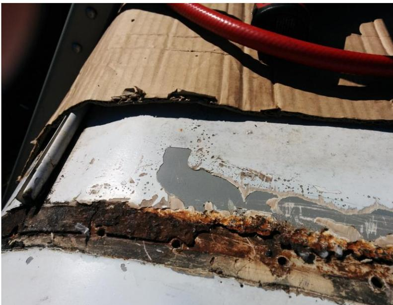
The exposed seam showing the state of corrosion.
